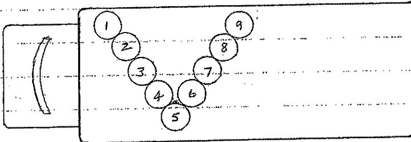
9-55gal. barrels in a V shape charge pattern
